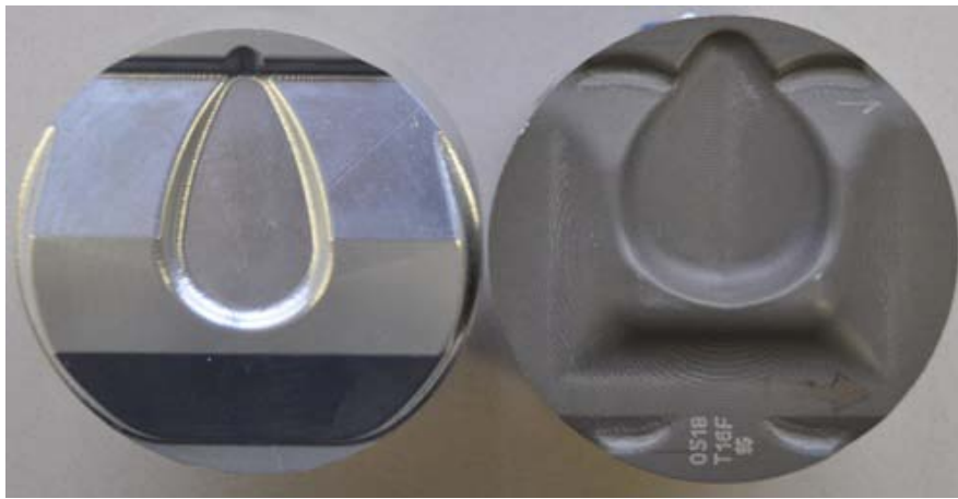
Fig.4.27 Picture of pistons for Injector A (Right) and Injector C (Left)
